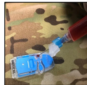
Figure A3 Loading cartridge sample well with blood
