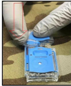
Figure A5. Sealing the cartridge
