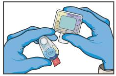
cHECK color of the indicator; if it is not similar to the "check" color on the reference scale (usually purple, with the exception of devices with a pull tab, which is usually a specific shade of blue), discard the unit and use a new one.
