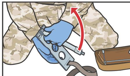
**07** **RAISE** the vertical arm up until it locks into place while simultaneously rotating it 90-degrees until the locking pin engages.
