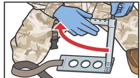
**08** **PULL** up on the vertical arm detent (retaining pin) and insert the horizontal arm. Release the retaining pin and advance the horizontal arm until the locking pin engages.
