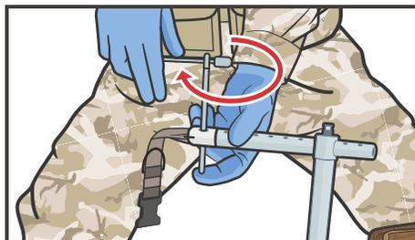
**09** **INSERT** the T handle into the horizontal arm and turn clockwise until it is threaded far enough to be stable and expose the end below the horizontal arm.
