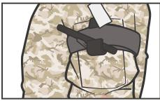
**ROUTE** the self-adhering band around the rod and between the clips.
