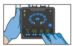
(b) Increase tidal volume. Using "Minute Ventilation Chart" with current respiratory rate (XX), increase tidal volume using the "up" arrow till the number reaches XXX and press "Confirm".
