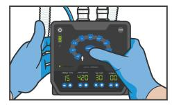
(a) Increase respiratory rate. Press the "up" arrow on the "Respiratory Rate" by two (2) breaths and press "Confirm"
