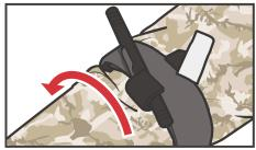
**ROUTE** self-adhering band around rod and between clips.
